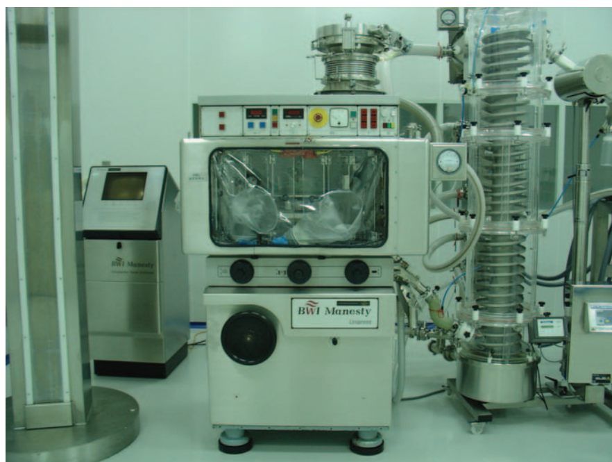
The isolator doesn't interfere with powder flow, tablet compression, or tablet movement.
